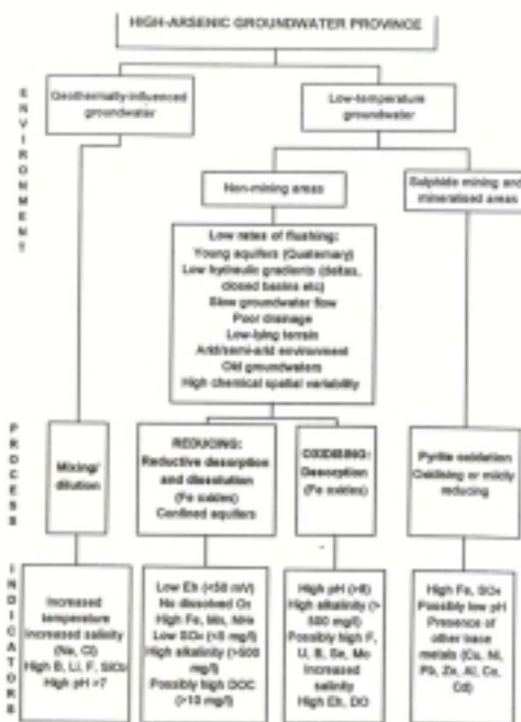
Figure 2. Flow diagram to assist identification of potential high-arsenic groundwater provinces (DOC; dissolved organic carbon, DO: dissolved oxygen. Eh: redox potential)
